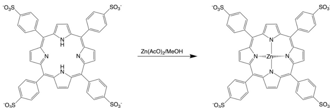
Fig. 1. Schematic for the \text{H}_2\text{TPPS}^{4-} (left) metalation with Zn to obtain ZnTPPS (right).
