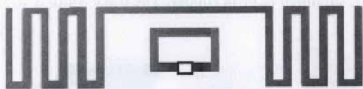
Figure 9b. A meander-line antenna with an inductively coupled loop feed.
