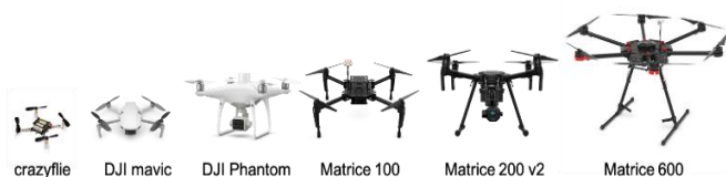
Figure 4. Some of the most used drone platforms. From left to right: a lightweight platform (crazyflie) to an industrial and professional platform (Matrice 600)
