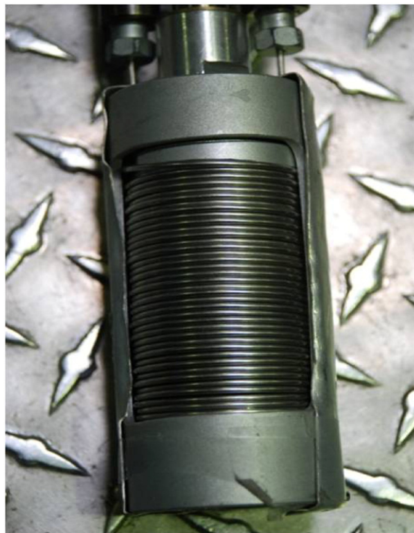
Fig. 1. High pressure cylindrical cell made from an inox capillary tube ( d_{int} = 0.5 mm, d_{ext} = 1.6 mm) enroled into an anular geometry ( H = 50 mm; D = 36 mm). The sample volume that can be illuminated by neutron beam is 1.3 cm 3 . The empty cell transmission is 0.75 at 2.23 Å. The cell has been tested to work up to 7 kbar.
