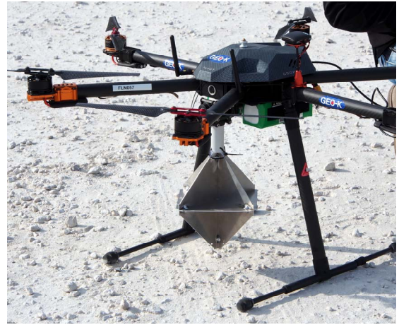
Fig. 13. Small size CR mounted under the drone’s body.
