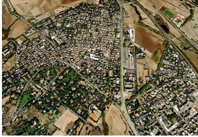
Figure 6.17: Aerial view of the simulation area. The figure shows the Google Earth aerial view of the simulation area. The related map in (Open Street Map) has been subsequently cropped and imported in Vanetmobisim in order to generate realistic mobility traces.
