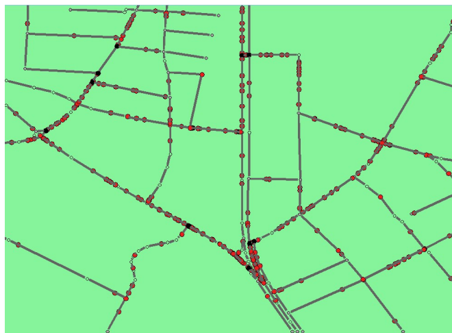
Figure 6.20: Realistic mobility pattern - Detailed view. The figure shows the situation of the mobility pattern generated on a real map, according to the IDM.LC mobility model (The red dots represent the constrained vehicles moving across roadmap during the simulation.).
