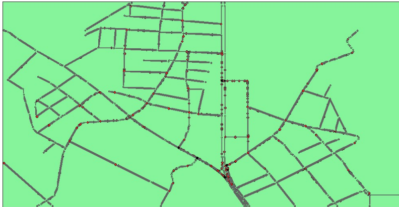
Figure 6.19: Realistic mobility pattern. The figure shows the mobility pattern generated on a real map, according to the IDM.LC mobility model (The red dots represent the constrained vehicles moving across roadmap during the simulation.). This trace has been used to compare CORP and CORP-TCP performances.
