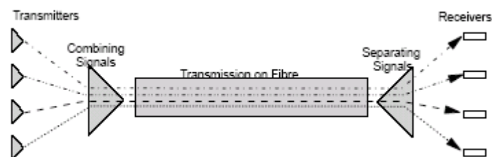
Figure 1.17 – Dense WDM (DWDM) scheme.
