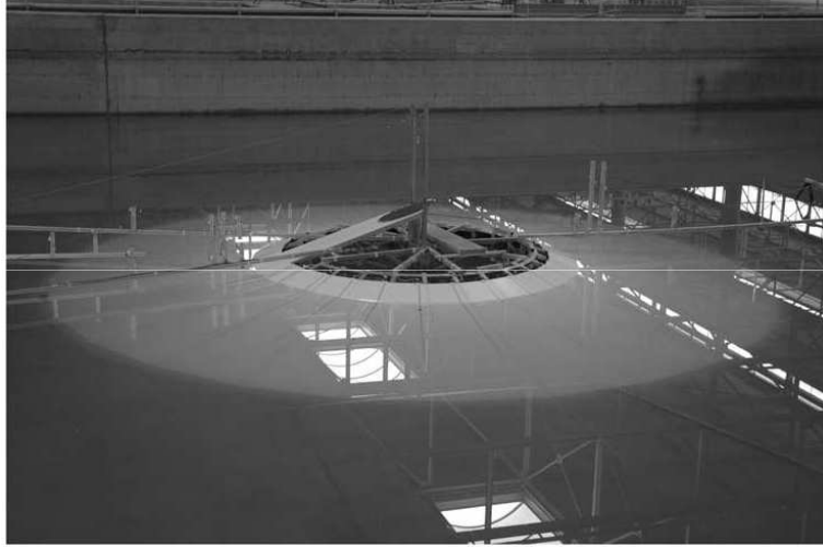
FIGURE 5.7: View of the experimental device used by Di Risio et al. (2009b). The landslide is forced to move along a plane incline 0.5 m wide; as a result the geometry of the experimental model is that of a very thin plane-beach strip connected to the curved flanks of a conical island.
