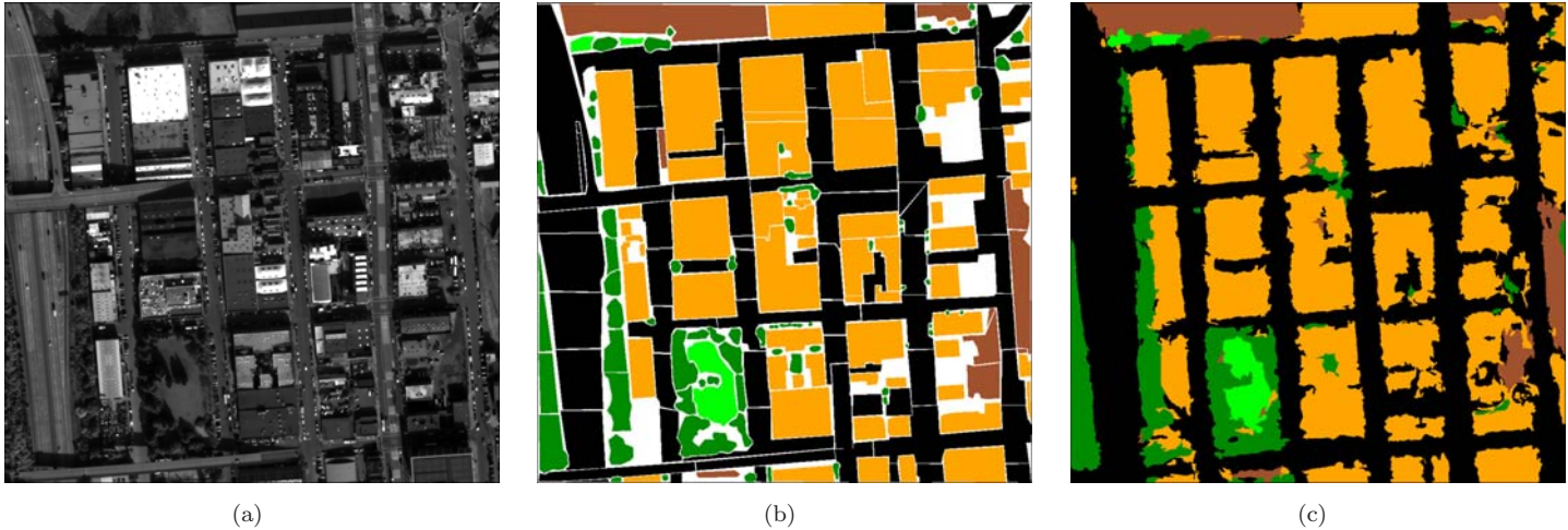
Figure 6.14: (a) Panchromatic image and (b) ground reference of San Francisco. In (c) is shown the classification map obtained using the reduced set of ten textural features. Color codes are in Table 6.6.
