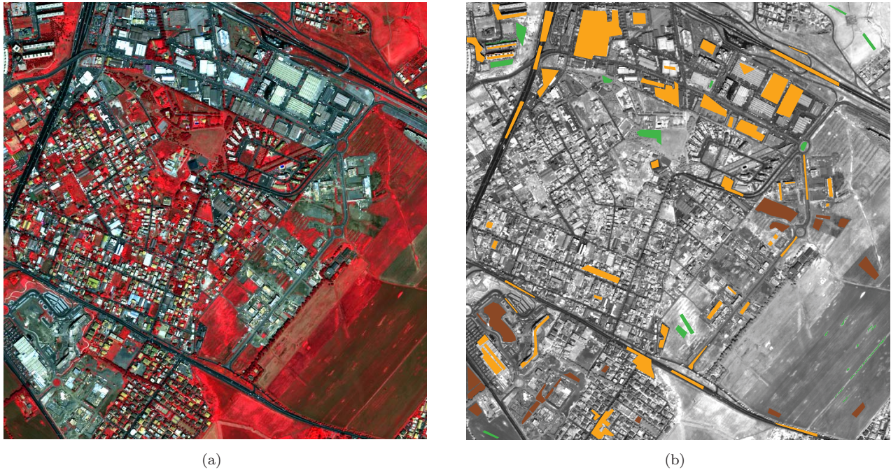
Figure 11.4: (a) Rome multi-spectral QuickBird image and (b) relative ground reference. Color codes in Table 11.2.
